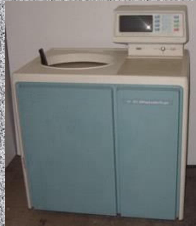
Ultracentrifuge can achieve 100,000 rpm with centrifugation forces of up to 802,400 g.
