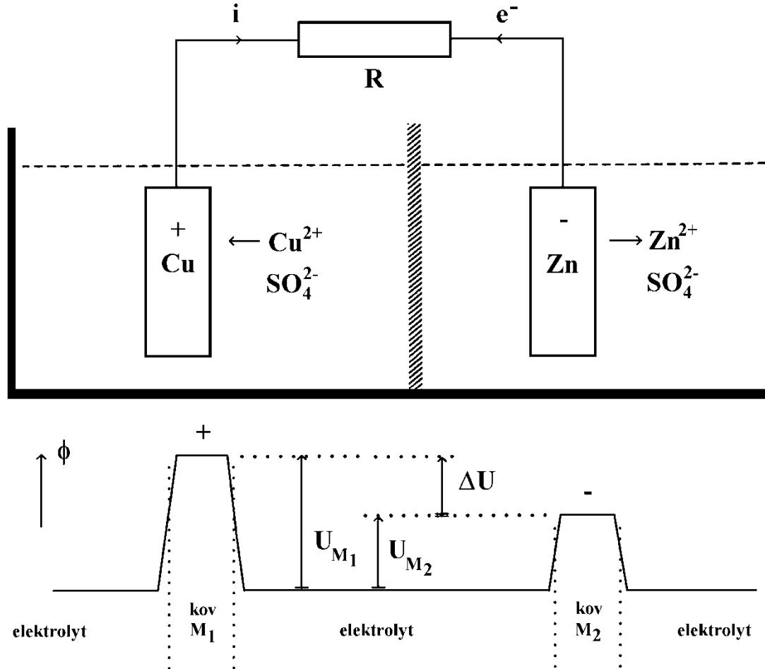
Origin of electric voltage  $U$  in the galvanic cell.  $R$  – working resistor,  $i$  – conventional direction of current,  $e^-$  - direction of electron flow. Down: Changing electric potential  $\Phi$  in the cell.
