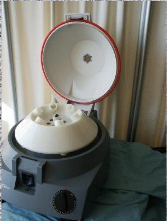
A small table-top centrifuge with open lid of the rotor space. Six positions for cuvettes (centrifugation tubes) can be seen.
