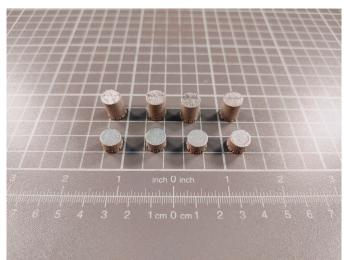
surface and in application of selected coatings in nano-layers with use of combination of these elements Ti, Si, Zr, Ag. We have developed the technology that provides promising parameters from the point of view of material science and should be evaluated in *in vitro* and *in vivo* tests.
